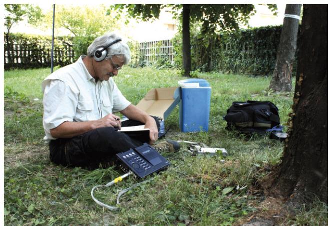
Figure 3: Michael T. Smith testing a sound detector at the base of a tree infested by CLB, Assago, July 2009.
