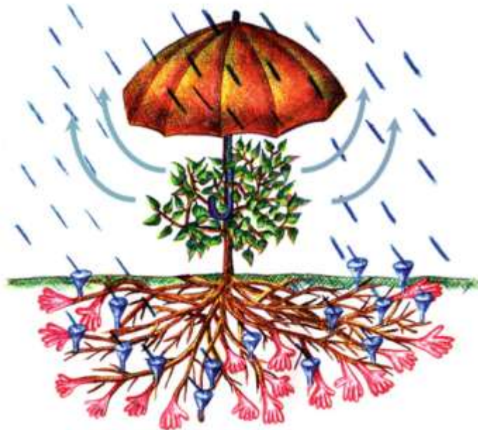
Figure 16. Soil stabilizing functions of plants, e.g. interception, evapotranspiration, and root reinforcement (Graf et al., 2019).
