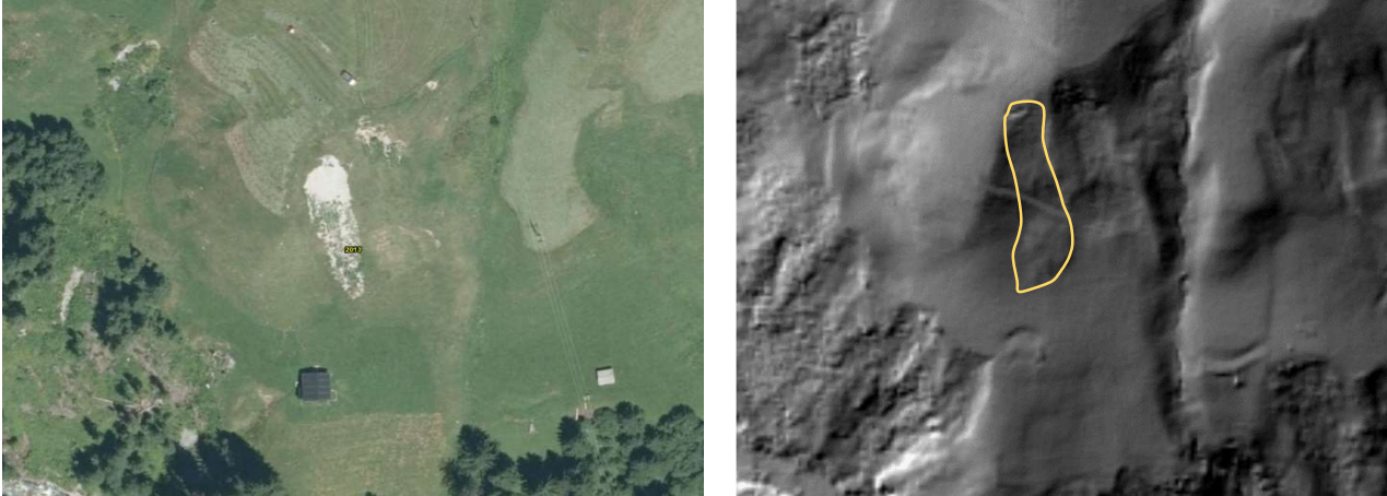
Figure 10. Example of debris/earth slide on orthophoto and digital elevation model hillshade. A debris slide leaves a clear negative imprint on the hillshade in the release area and positive imprint of the deposit, while debris/earth flows are often not recognizable on hillshades.
